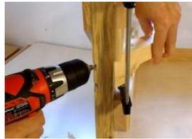
Then you can countersink a 2” wood screw to hold the side panels in place. Do this on top and bottom (all four holes per side panel).
